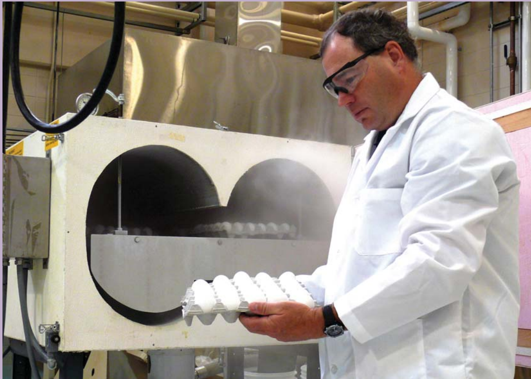
Kevin Keener developed a rapid egg cooling system that uses circulated carbon dioxide to create a thin layer of ice inside an egg's shell that cools the inside of an egg within minutes. (Photo by Keith Robinson, courtesy of Purdue Agricultural Communication)
