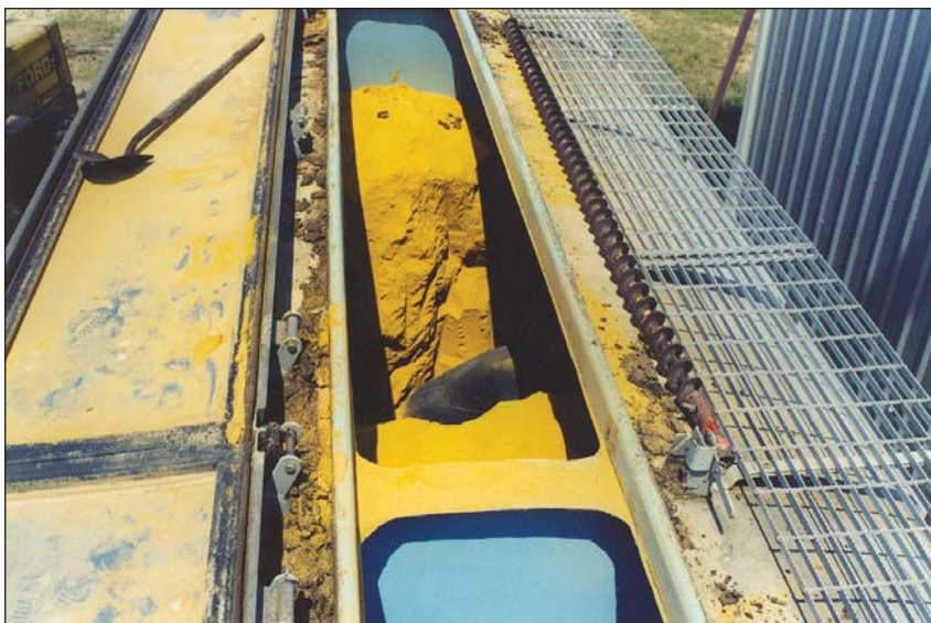
The use of manual labor to unload a railcar caked-up with DDGS is not only time consuming and expensive, but it is also risky.
